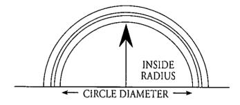
For an Arch (or Eyebrow), provide the width and the rise in the center of the curved portion.
