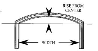
Elliptical curves require a template. The template may be drawn on paper or cardboard. WOOD TEMPLATES ARE NOT NECESSARY.
